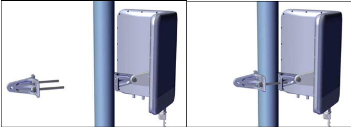
Figure 14: Second radio holder fastened to a MultiSector unit
