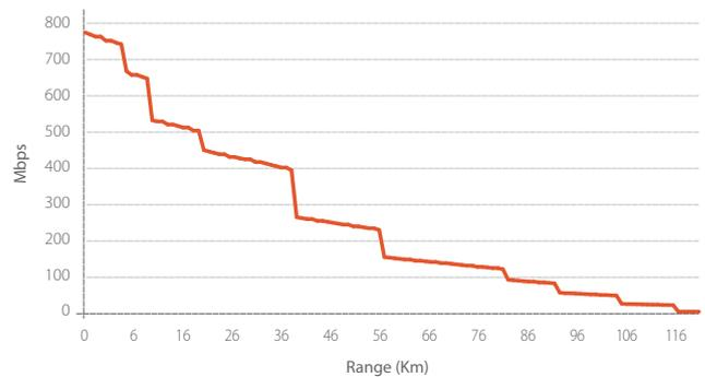
\* 5.8GHz, 80MHz, 32dBi antenna
