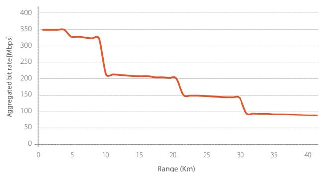
\* 5.8GHz, 80MHz, 22dBi antenna
