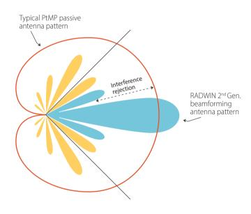
JET DUO 5 GHz beamforming antenna pattern vs. a typical PtMP antenna
