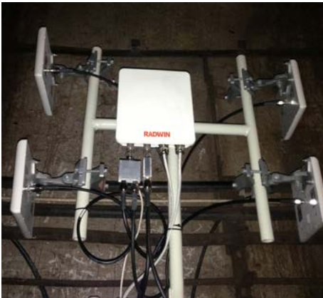
FiberinMotion® base stations and mobile units deployed along the tracks and on the trains
